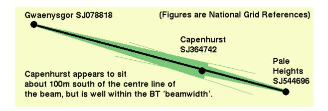
It is also located right on the microwave line-of-sight between two British Telecom radio towers at Gwaenysgor in North Wales and Pale Heights in Cheshire.
